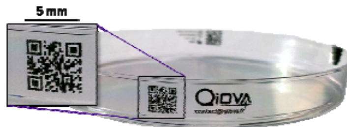
Figure 3: Alphanumerics and 2D code marking inside the rim of a crystal Polystyrene Petri dish
