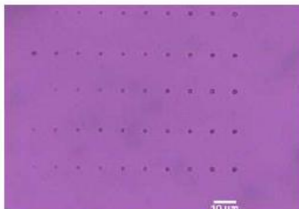
Figure 9: micron scale holes drilled in BK7 with increasing energy
