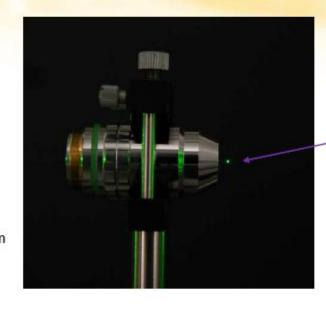
Stable optical breakdown in air
